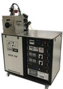
**Magnetron Sputter System with RF Power Supply**
